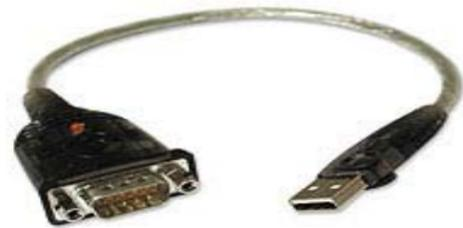
**IOGear USB to Serial Adapter** - One end fits in an available USB port on your computer and the other end is a standard 9-pin serial which connects to your real-time cable or to a cable attached to the viewer's computer.
